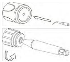
\*To remove sclaer handpiece from tubing, Gently pull straight off. Don't turn / twist or damage to tubing pins will occur.
